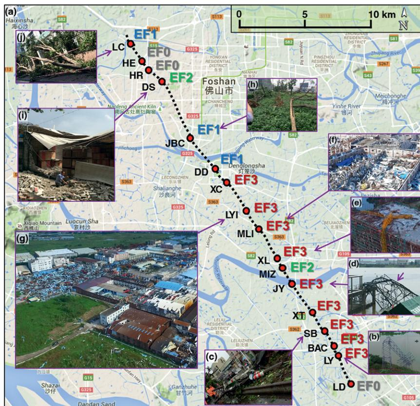
**FIG. 2. (a) Tornado track (black dashed line) with rated EF scales at some detailed ground survey sites (red dots) mapped onto the Google map. (b)–(j) On-site damage photographs at some locations along the tornado track. North is indicated by a white arrow in the upper-right corner.**
