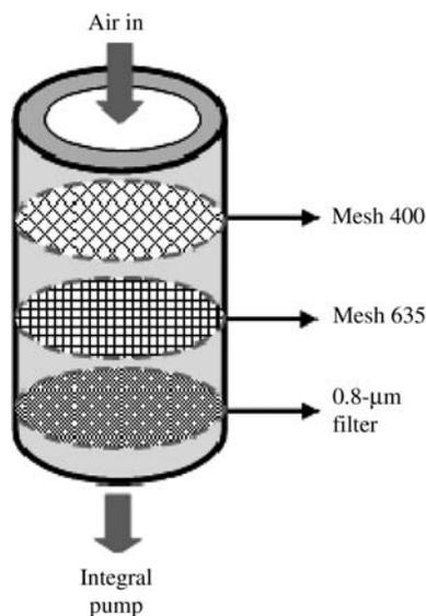
Figure 1. The diagram of the screen array for  $^{212}\text{Pb}$  particle size distribution measurement.
