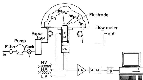
Figure 1. The electrostatic radon monitor (ERM).
