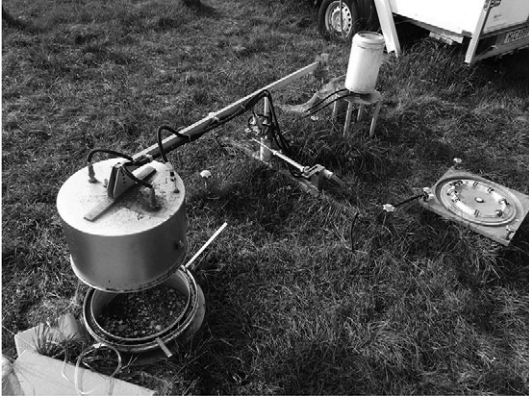
Figure 1. Exhalometer set-up in operation.
