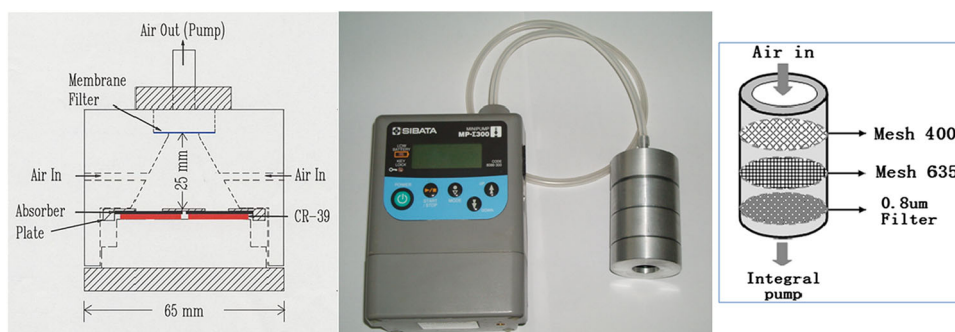
Fig. 1 The drawings of thoron progeny concentration and size distribution measuring devices
