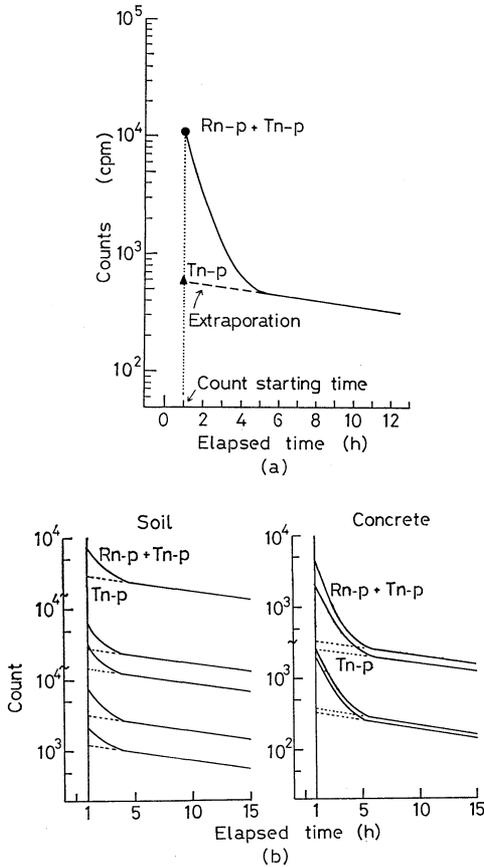
**Fig. 1(a)** Decay curve of Tn and Rn progeny on the sampling filter, Tn-p: Tn progeny and Rn-p: Rn progeny.
