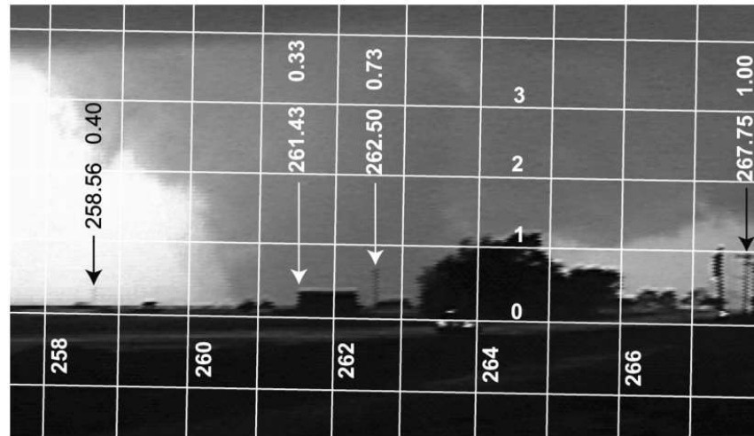
FIG. 3. Image of the Dimmitt, TX, tornado of 2 Jun 1995 obtained by the "CAM-1" VORTEX intercept team using Super-VHS video. The four survey landmarks are marked with arrowheads near the survey point, and azimuth and elevation notated in decimal degrees. From left to right, the landmarks are a faint power pole, the left roof peak of the barn, a power pole to the right of the barn, and the top of the second power pole from the image edge. The Cartesian grid overlay was generated in graphics drawing software and magnified, translated, and rotated to find a subjective best fit with the survey data.
