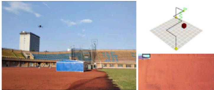
(a) The UAV detects the private region and re-plans its trajectory and camera orientation.
