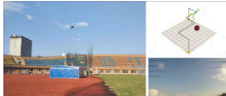
(b) The private region is avoided by changing trajectory and camera orientation is tuned to 30^\circ .
