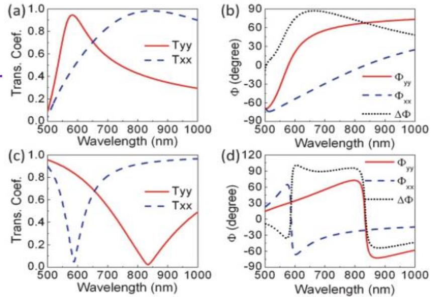
FIG. 2. (Color online) (a) Amplitude and (b) phase of the transmission coefficients for linearly polarized excitations for the optimized metasurface geometry of Fig. 1. (c, d) Similar plots for the complementary geometry, composed of plasmonic nanorods.
