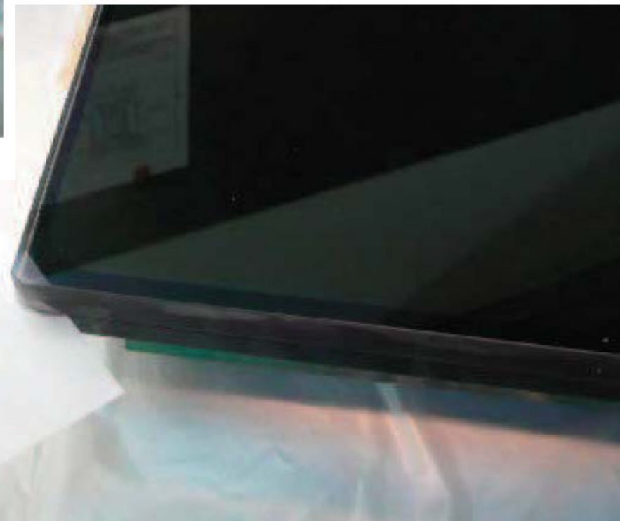
Fig. 2.— The last mylar shim in place while gluing the u filter
